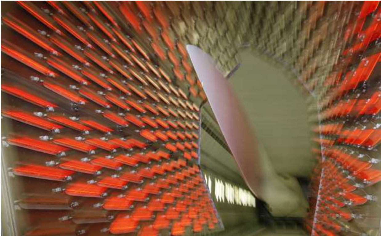
Rotor blade manufacturing for wind turbines by Nordex in Rostock, Germany
